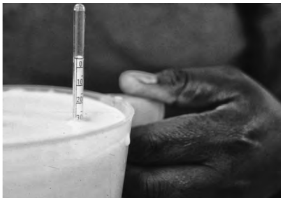
FIGURE 12 Using a lactometer to test milk for adulteration in Kenya's informal market.
