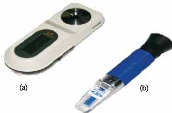
Photo 2.30 Refractometers for measuring total soluble solids in °Brix: (a) digital model, (b) sight glass type
