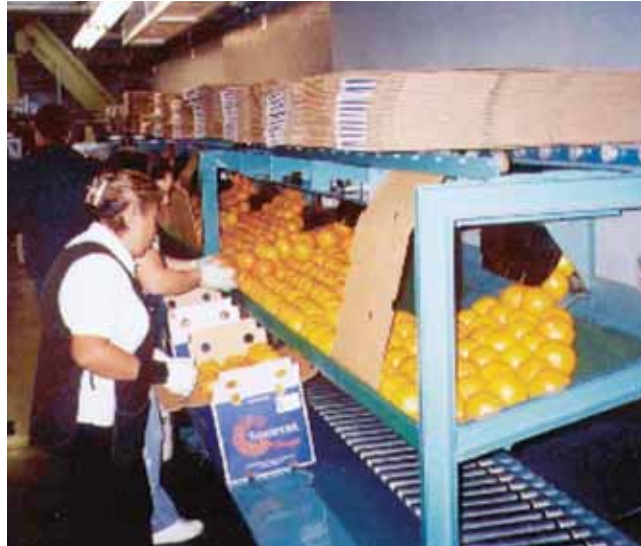
Photo 2.17 Packing of citrus in cartons. The work area is divided into three levels: the top level has a conveyor for packaging materials; the middle level accepts fruit from the preparation area and presents it to the packer at a convenient height and within easy reach; the bottom level accepts filled cartons and conveys them to a dispatch area
