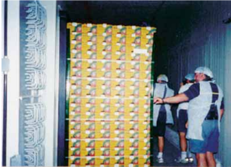
Photo 2.11 Forced air cooling of Brazilian mangoes packed in fibreboard cartons
