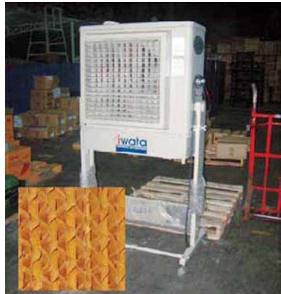
Photo 3.2 An evaporative cooler that makes use of cellulosic pads (inset) as wetted media
