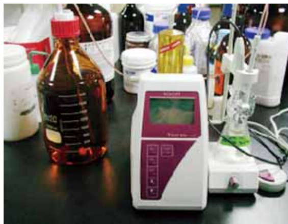
Photo A.2.2 Autotitrator for determination of endpoint at pH 8.2 using 0.1 N NaOH solution
