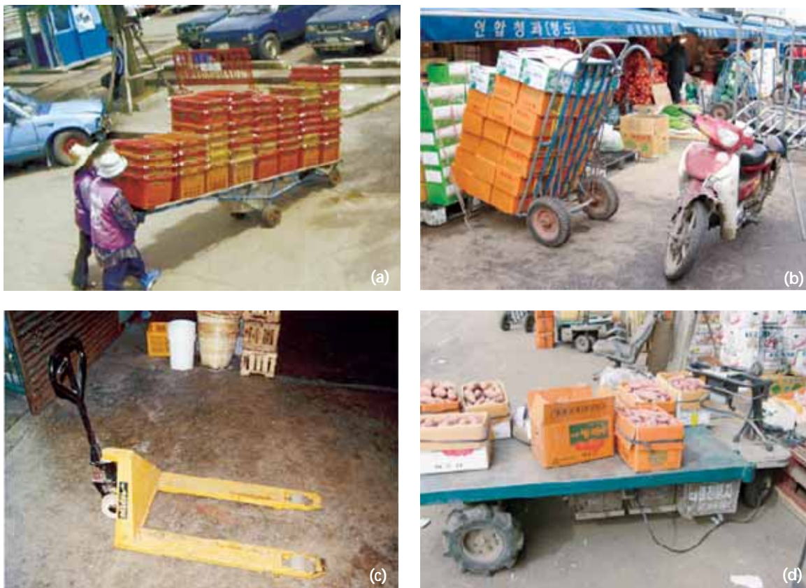
Photo 2.26 Types of carts and forklifts used in pack-house operations in developing countries: (a) fruit baskets loaded on a four-wheeled cart; (b) vegetable cartons on a two-wheeled cart; (c) manual forklift, also known as a pallet jack; (d) electric cart powered by rechargeable car batteries
