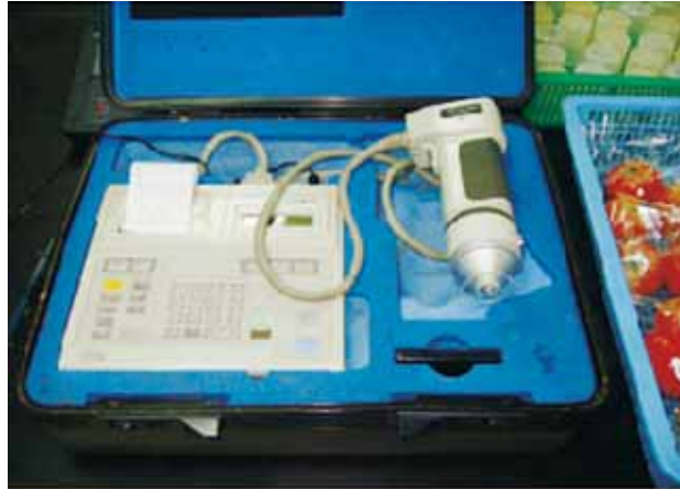
Photo 2.29 A chromameter for measuring L^*a^*b^* values of fruit and vegetable samples
