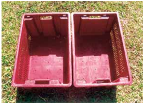
Photo 3.1 A plastic crate design that is both stackable and nestable. In the position shown, the right crate can be stacked on top of the left crate. If the right crate is rotated 180°, the two crates can be inserted into each other
