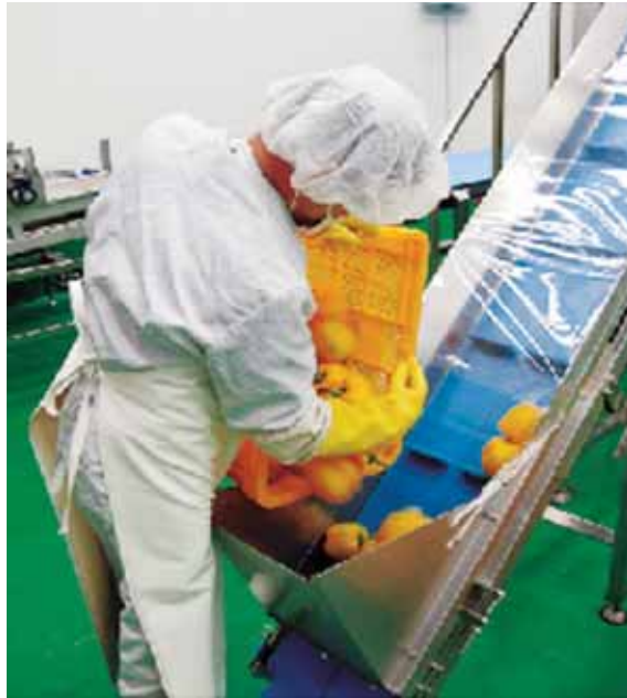
Photo 4.1 Protective garments for personnel in a pack-house facility. Each worker is fitted with a hair net or cap, gown, thick apron and gloves, and boots. All garments are white for easy detection of contamination
