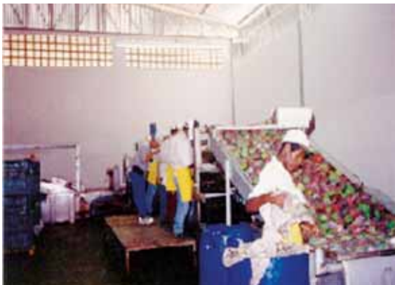
Photo 2.4 Washing of mangoes by immersion dipping
