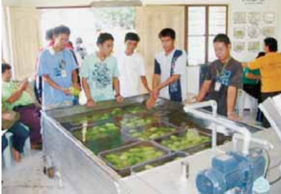
Photo 2.23 Demonstration of hot water treatment of mango (left) for post-harvest disease control to a farmers' cooperative. Water temperature should be monitored carefully with an accurate thermometer to avoid heat injury to produce (right)
