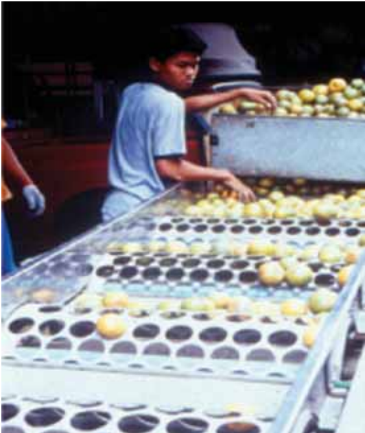
Photo 2.21 Perforated cylinder sizer for citrus makes use of rotating steel cylinders with successively larger openings to classify fruits according to diameter
