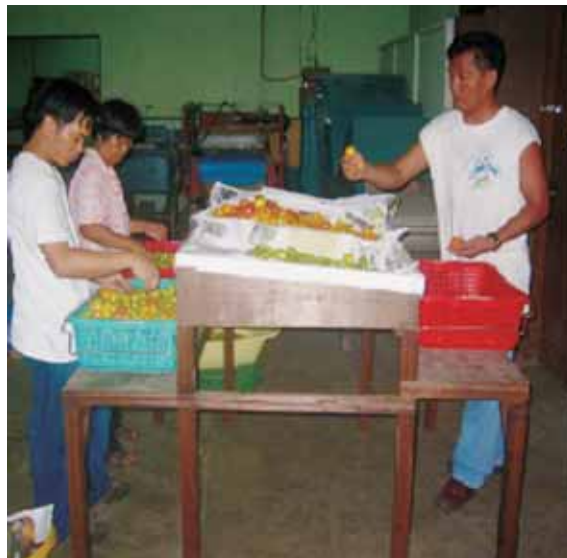
Photo 2.19 Prototype sorting table being tested for tomatoes. Fruits of mixed ripeness (left) are sorted into different compartments (middle) according to peel colour. A packer (right) places sorted fruit into individual cartons according to peel colour
