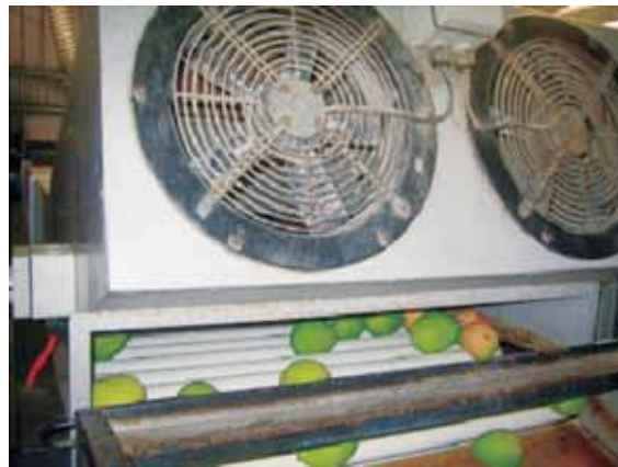
Photo 2.24 An air dryer equipped with blowers and a roller conveyor for evaporating surface moisture from mango fruit
