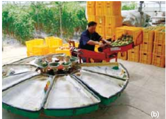
Photo 2.22 Weight sizers for mangoes (a) and tomatoes (b)
