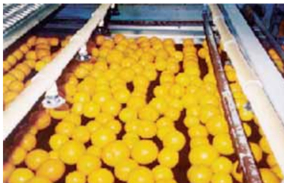
Photo 2.6 Waxing of citrus by spraying
